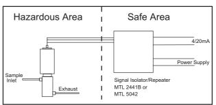
**Note**: Samples should be taken from the upper surface of the main line to prevent any risk of condensate reaching the sensor. Additional components may be required for specific applications - refer to *Accessories* and *Sampling System* specification sheets. Use stainless steel, nickel or copper piping wherever possible.
