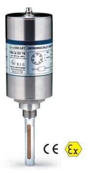
The Alpha Moisture Systems **Model ADHT-Ex** is a 3 wire, 4-20 mA, 24V powered dewpoint transmitter. The unit is fully self contained in a robust stainless steel casing with weatherproof protection to IP65, making it ideal for use in heavy industrial environments.
