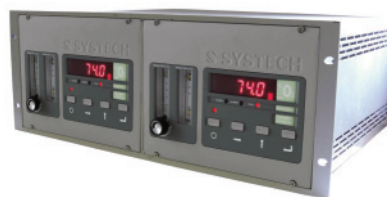
Rack Mount 4U - 19 inch Houses 1 or 2 Analysers 178H x 484W x 410D (mm) 9.7kg (single unit)
